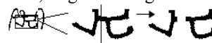
Fig.7: Joined characters separated using VPPs For connected character again the procedure of VPPs is applied, ignoring the headline, and segregation is made starting from the middle of the connected characters and moving in both the directions, looking for minimum value of VPP, for making the cut. If traversal in both directions leads to extreme ends then either the characters are connected at more than one points or they are merged.
